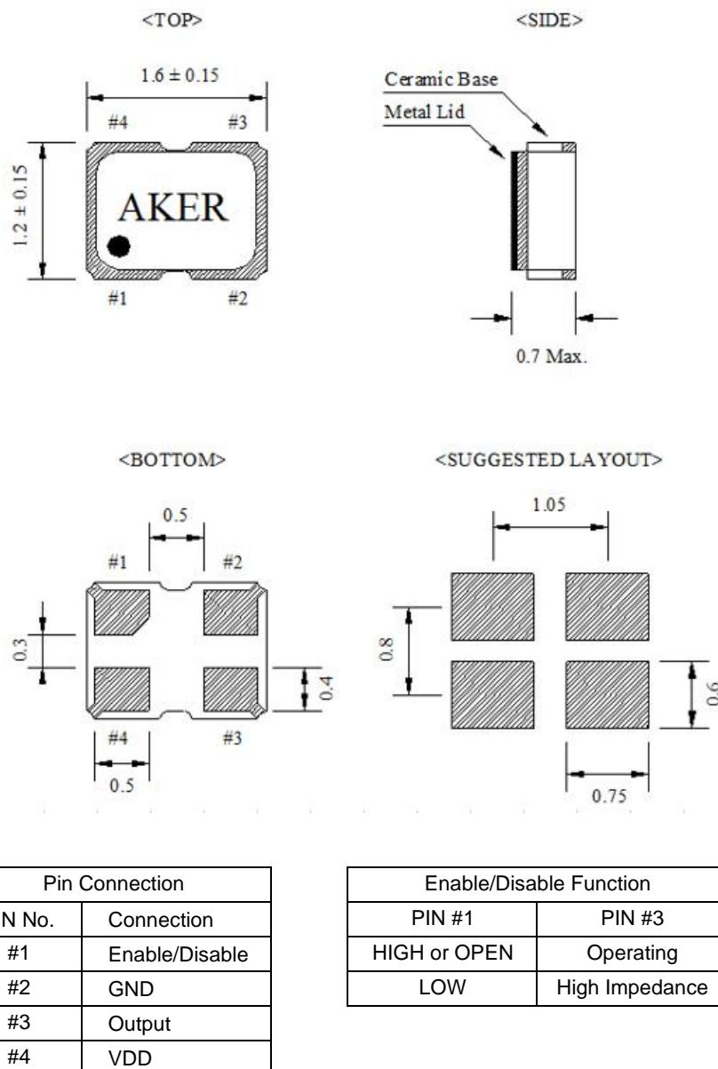
Package is Seam Sealed Ceramic-Metal.
